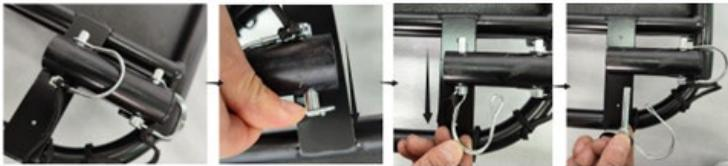
Then push the tow bar into the tube provided on the left side. Secure the inserted tow bar with the two quick release pins. The elbow of the tow bar is now pointing to the right in relation to the direction of travel. *Important: Make sure that the pin is securely locked, as a loose tow bar could cause you to lose control of the trailer while driving.*
