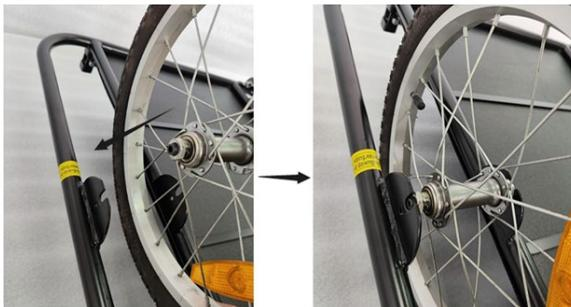
Then fit the parts marked "inside" to the quick-release cylinder and tighten it. Proceed in the same way on the opposite side with the other wheel.
