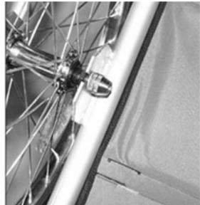
Take a wheel and position it in the guide provided in the frame so that the lever of the quick release cylinder is on the outside of the trailer.
