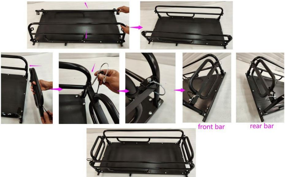
1. Unfold the trailer frame and remove the wheel guards;
