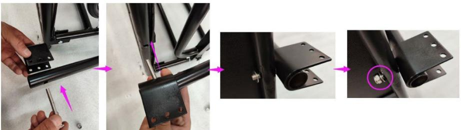
Assemble the upper part of the tow bar using the screw and wing nut in the
