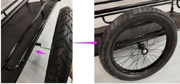
Place the wheel axle in the frame tube and make sure the wheel is properly locked.
