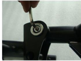
4. Install the damper(6) on the loading frame(1) as per below images :
