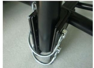
6. Install the coupler under the seat post as per below images:
