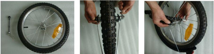
3. Connect loading frame(1) and the fork with wheel by connect nut(10) as per below images:
